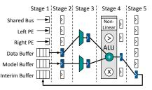
Figure 6: Pipelined PE. Black highlights an Add operation (Interim-Buffer[i] = DataBuffer[j] + ModelBuffer[k]).
