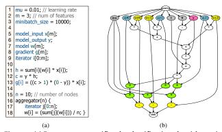
Figure 4: (a) Programmer specifies the classification algorithm as its gradient and aggregation functions. (b) Translator outputs the DFG.
