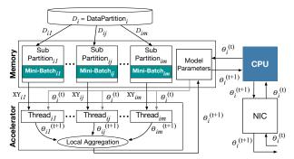
Figure 1: Execution and acceleration flow within each node.
